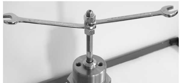
Figure 6 Handle Construction for Lapping
