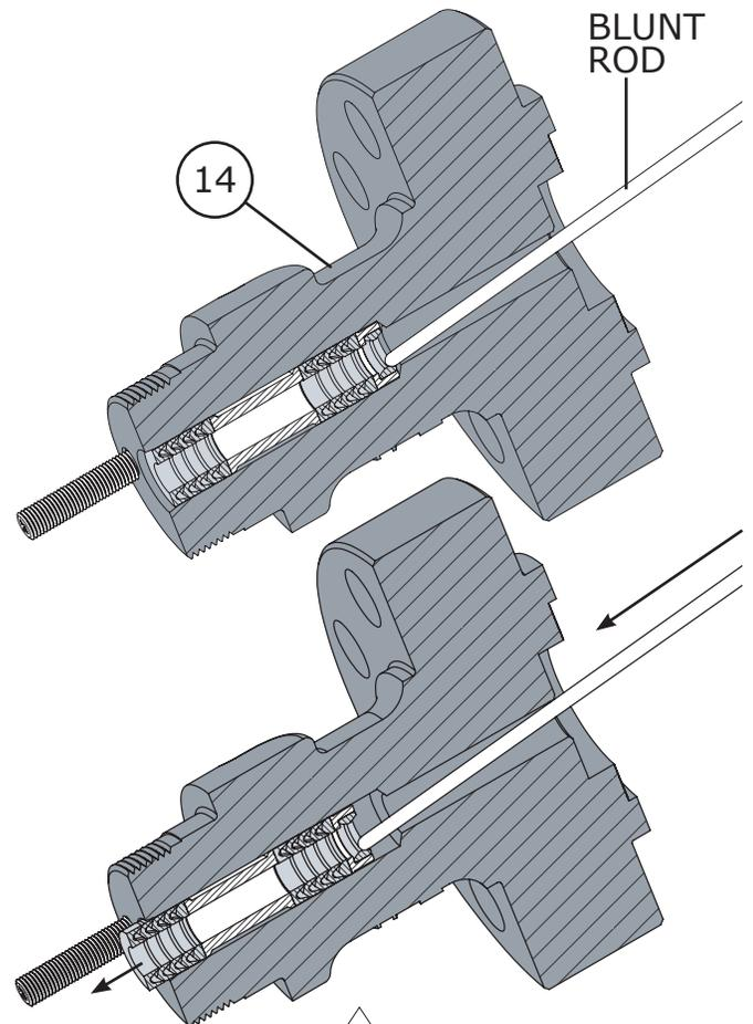
**Figure 13** Packing Parts Removal (Step 1)
