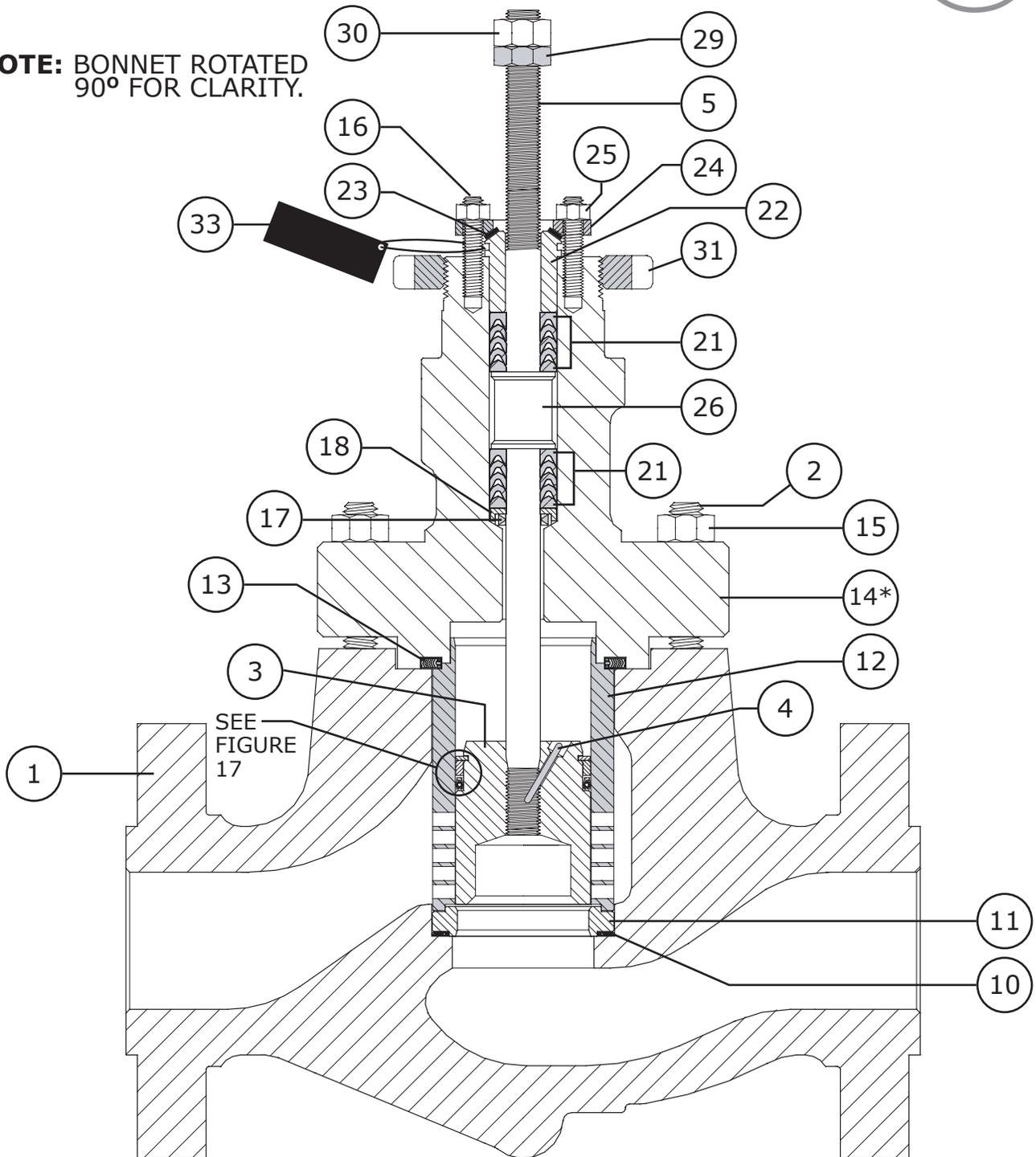
**Figure 31** Model 390 Control Valve Cross Section
