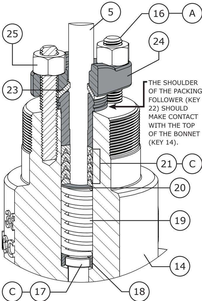
**NOTE: SILICONE-BASED O-RING COMPOUND (KEY C) SHOULD NOT BE USED WITH OXYGEN SERVICE.**
