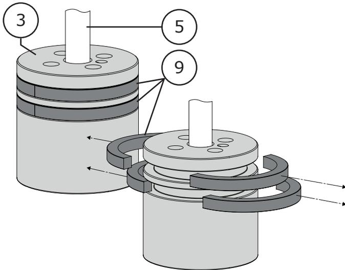
**Figure 11** Model 391 Piston Ring Removal
