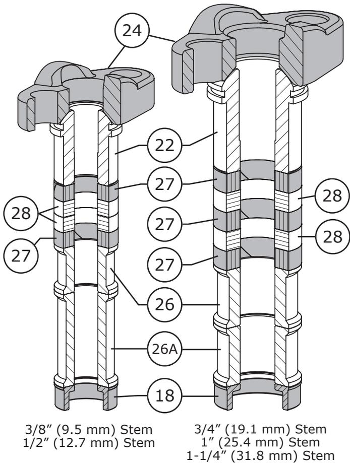
**Figure 29** Single Graphite Packing Arrangement
