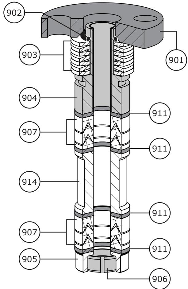
**Figure 30** Live Loaded Packing Example
