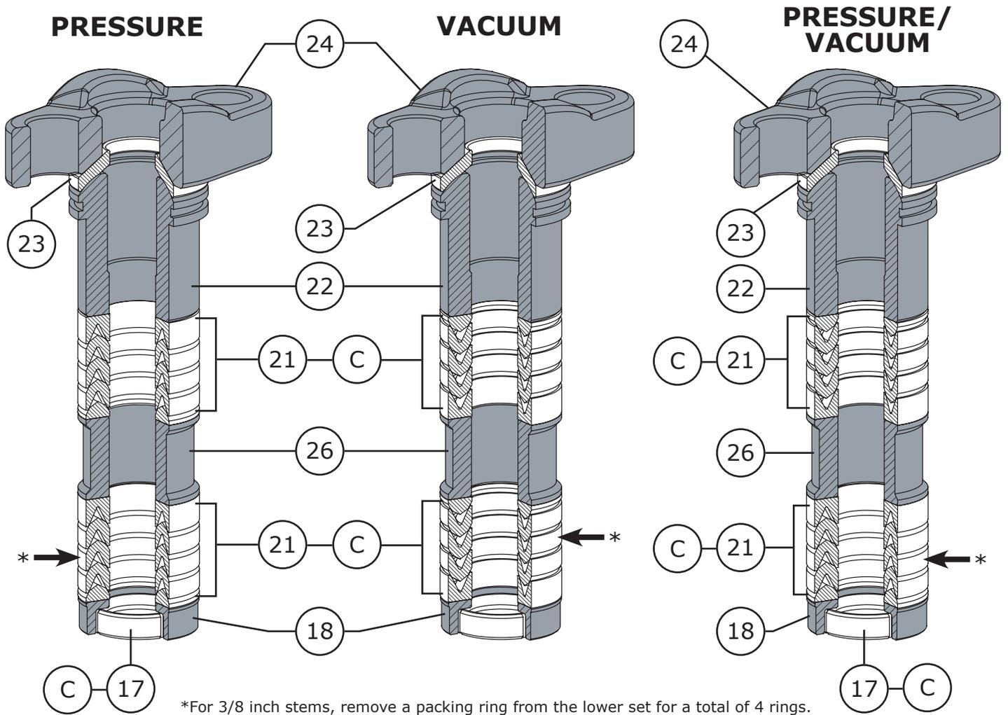
Figure 28 390 Series Control Valve PTFE Packing Diagrams
