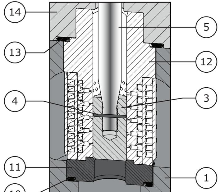
**Figure 36** *Anti-Cavitation Trim Detail*
