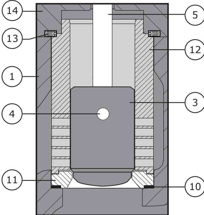
**Figure 12** Model 392 Plug Diagram (Refer to Figures 36 to 39)
