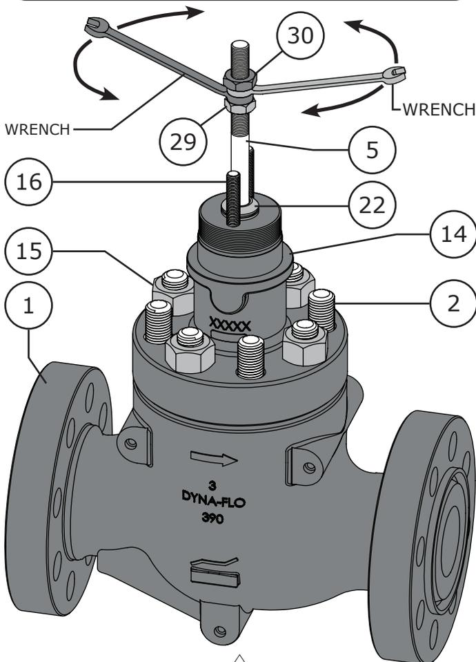
**Figure 16** Lapping Procedure Setup (Steps 9 - 10)
