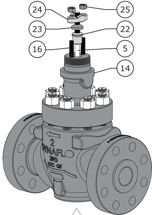
Figure 6 Packing Removal (Steps 1 - 3)
