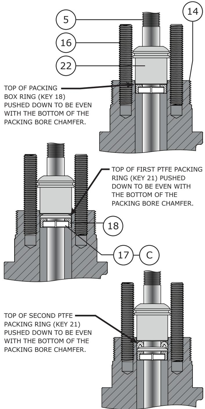
**Figure 25** Proper Packing Ring Installation
