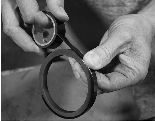
Figure 18 Piston Ring Assembly for Model 371 Valves (Step 1)
