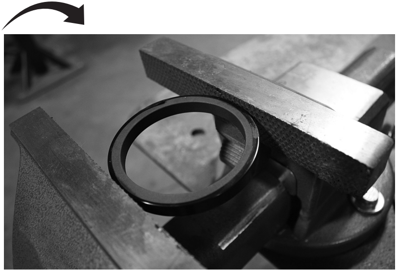
Figure 19 Piston Ring Assembly for Model 371 Valves (Step 2)
